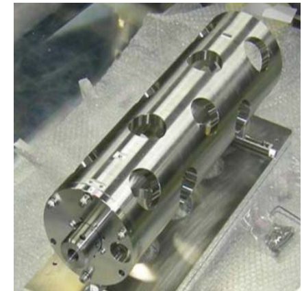
Pulse stacking cavity L_{cav} = 420 mm
